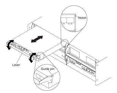
Figure 78. Installing a controller
